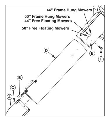
Figure 14. Install Middle Tube
